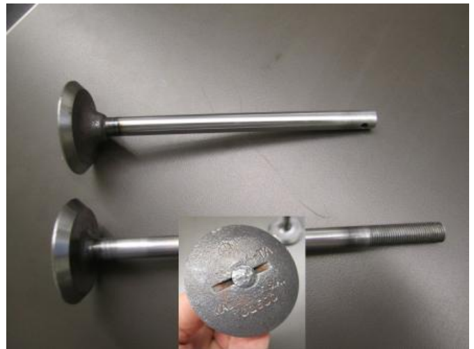
Ron Gerlach replaced the stems on these valves. Inset: top of stem peened to lock valve's head to stem.
