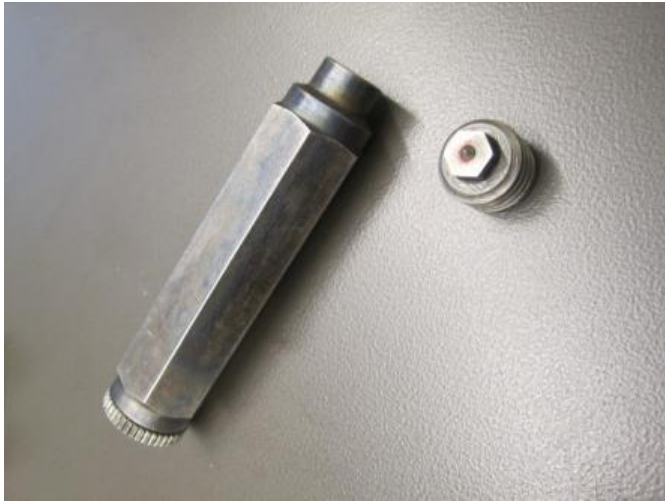
Transfer punch set. Handle (L) has a hex socket on one end to turn punches (R.) Handle is hollow, enabling storage of multiple punches of the same size.
