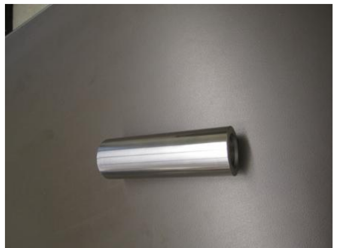
Ron Gerlach made this wrist pin from a length of linear shafting.
