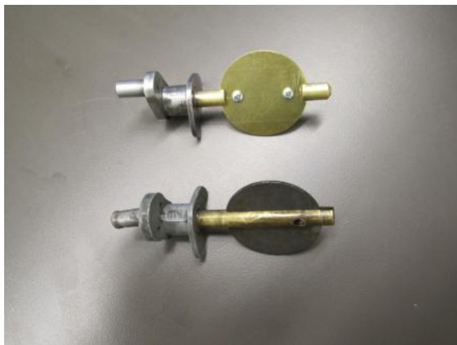
Ron Gerlach made a replacement butterfly assembly (Top) for his IHC Model M engine.
