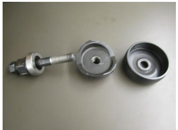
Eldon Barkley modified this Greenlee knockout punch by cutting threads farther up its shank.
