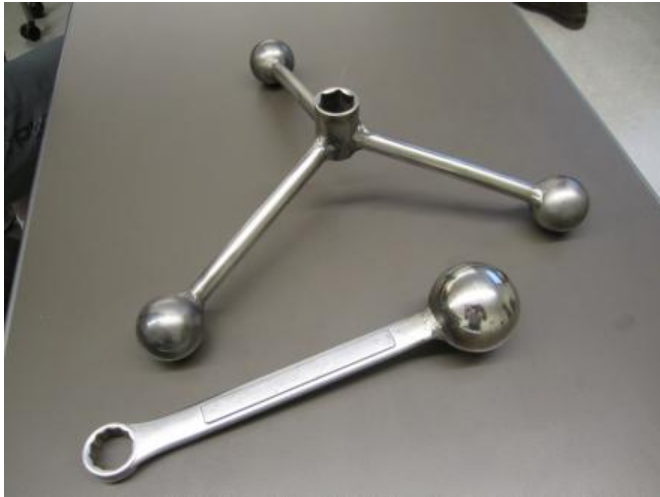
Matt Rulla's home-made vise handles. Lower: Original design. Upper: Speed Handle.
