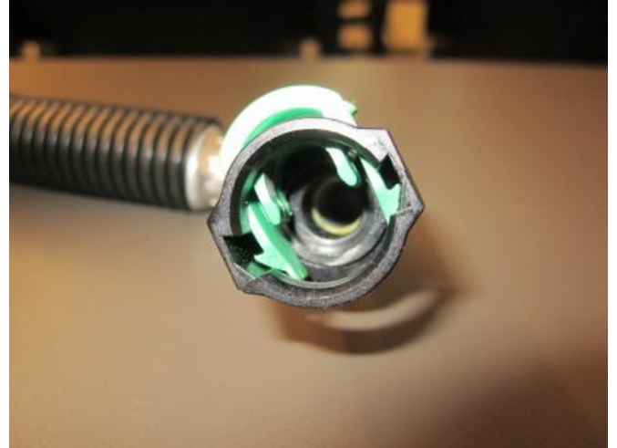
A quick coupler from Millar Farewell's Polaris side by side buggy. An o-ring deep inside needed to be replaced without being damaged.
