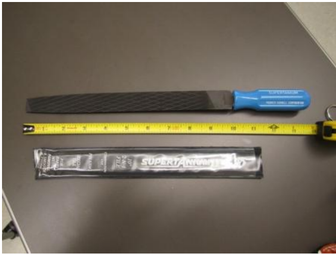
Matt's "Supertanium II" file. The coarse side is facing up and has a waffle pattern to help clear the shavings.
