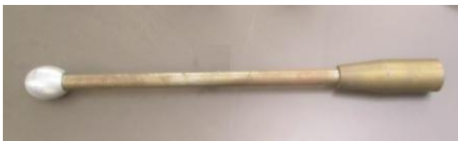
Eldon's tool for removing stubborn centers from his lathe's spindle.
