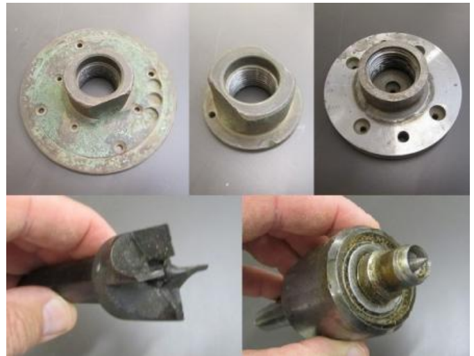
Top Row: Three woodturning faceplates. Lower L: Spur Center. Lower R: Cup type live center.
