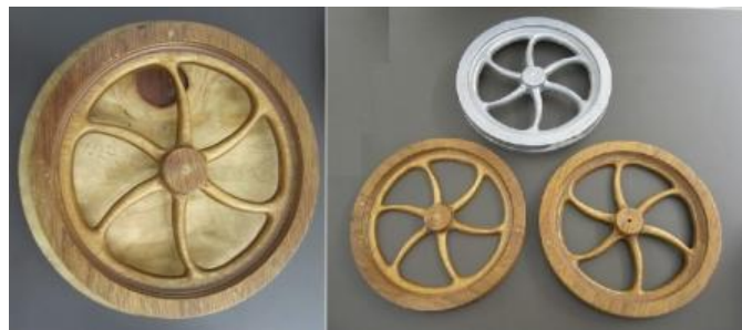
L: One half of Eldon's split pattern sitting atop a sacrificial plywood mounting plate. R: Complete split pattern with flywheel casting.
