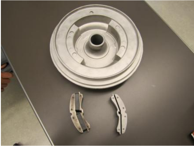
Top: Bob DeVoe's problem flywheel with magnets inside the casting, near the inner diameter of the rim. Bottom: Magnets
