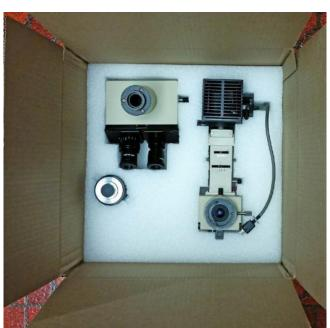
He first had to disassemble the heavy unit into manageable sub-parts and made custom compartments for each piece. He utilized sections of Polyethylene foam inside of double wall cardboard boxes to form the protective cavities. These boxes were obtained from Box Zero, a supplier of packaging supplies, located in Orange on Katella.
