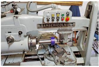
preparation for any of these gear cutting operations. The hobbers have drive spindles for both the cutters (hobbers) and the gear blanks. These spindles need to be synchronized with a series of change gears for proper operation.
