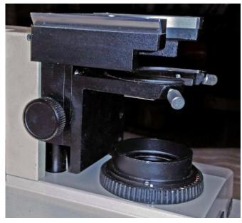
This microscope had been shipped to Larry's residence and was well packed for shipment but apparently the previous owner left the condenser assy in mid position before shipment and the weight of the part combined with the usual vibration and shocks of shipment resulted in a damaged rack where it was mated to the elevating pinion gear. The rack was made of a
