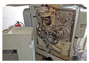
there is also a necessity for absolute minimal backlash in the change gear trains. Mr. Cruz explained some of the details during the tour. Besides the actual gear hobbing machines there
