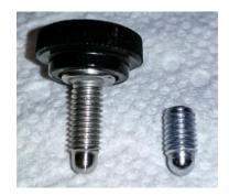
carbide form tool rather than a traditional radius cutting fixture. He had a series of quarter round form tools from Micro100 and had one with a radius that was close enough to be use for the application.
