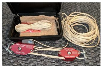
This locking mechanism can support the full 750lb weight capacity of the system. Being a 4:1 lever system, the lock only has to withstand 1/4th of this weight. There are videos on Youtube of users stressing these Nifty-Lifts to twice their rated capacity of 750lbs so there is a healthy amount of over design in the product.
