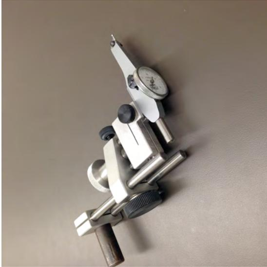
England. This tool is in remarkably good shape for being a vintage tool. It reads the same direction on the dial no matter which way the probe is moved. Next Norm showed a Federal dial test indicator and talked about how to setup the tool for maximum accuracy. Norm showed three or four other types of indicators and mounts, including a shop made "Zero It" clone.
