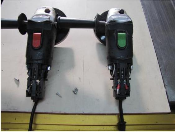
intermittently when the power chord was moved around. Both were diagnosed with the same problem of a broken wire at the rear of the tools where the power chord entered the motor
