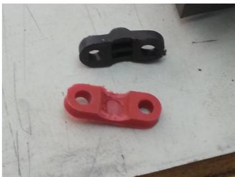
Before replacing the clamp, he filed out a bit of material under the clamp piece.
