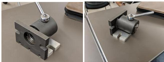
There was also a nice American made collet in the closer at the time he found it. He was asked how he managed to find this nice tool in a trash can but there was no clear answer. To improve the tool, Norm added an additional plate to make it mountable in the Horizontal position as well as the original Vertical mounting.
