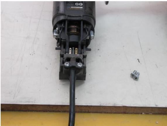
body. Apparently, the clamps holding the wires were just too small and severely deformed the chord underneath resulting in broken wires. His fix was to merely cut off the chord at about the entry point, strip a fresh length wire and to crimp on new lugs.
