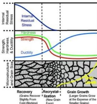
Next up was a discussion of the Grain Growth vs Temperature chart. This chart is for steel with varying amounts of carbon and no other alloying elements or compounds added. During cooling,
