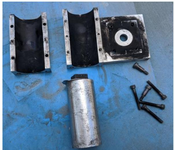
After the Babbitt cooled down it was placed in the lathe, on a special mandrel, and turned to the correct OD. This operation required the center form to remain in place in the raw slug.
