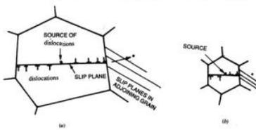
Fig. 2.16 Pile-up of dislocations against grain boundary in (a) Coarse grained material, (b) Fine grained material.
