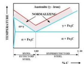
Annealing is achieved by heating the steel up past A3 and soaking (The soak time would be a function of thickness); then cooling slowly by leaving the steel in the oven and allowing the oven to cool by itself. Normalizing involves multiple cycles of raising the steels temperature to just above A3 (by approx.. 50 degrees C) and then
