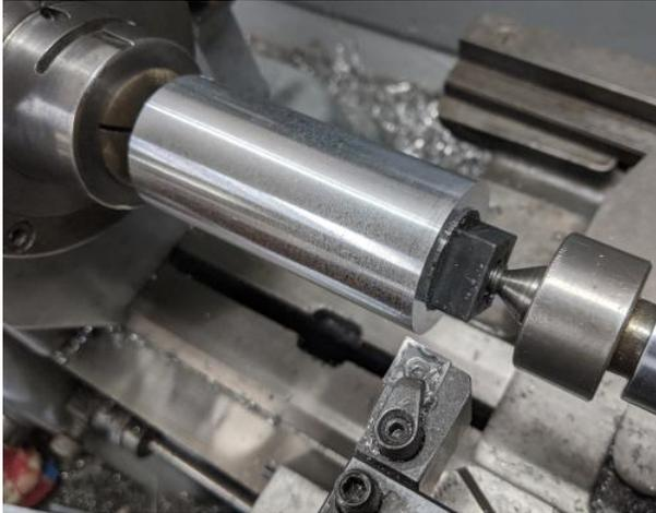
The finished shell is shown below. After this point it was pressed into one side of the engine crankcase casting and then the grease flow tracks were cut by hand. These tracks allow grease to flow from the grease entry point along the length of the bearing.
