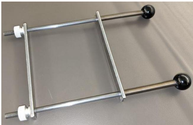
sliding cross piece. The two cross pieces would be placed within the jaws of the vise, pressing outward on the parallels, thus keeping them firmly in place as the jaws are moved.
