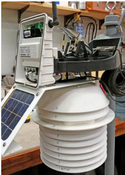
cells during daylight hours. At night the fan runs on the charged NiCad battery and the electronics run on the charge in a supercapacitor. This constant flow of ambient air means there is an accumulation of stuff inside the unit. He had to do a complete tear down of the enclosure to perform a proper cleaning, which he repeats every 18 months. He took multiple photos during this process to aid with assembly. He was
