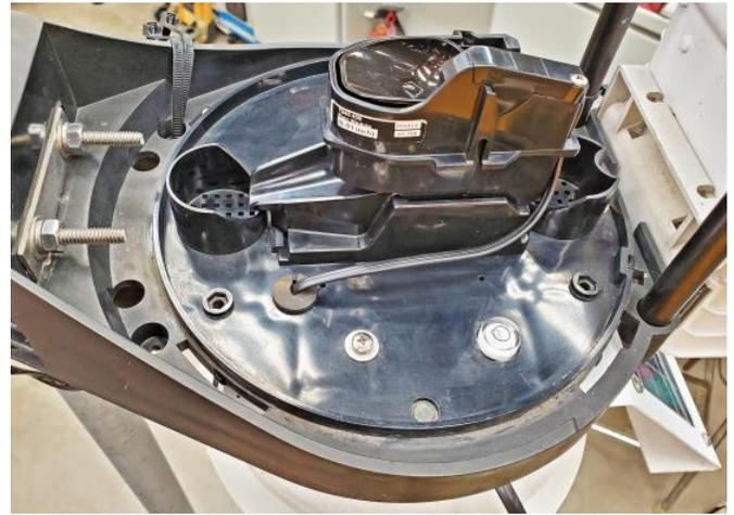
sharing these photos and giving the club a glimpse of the internal workings of the unit. The above image gives a partial view of the tipping bucket mechanism used for metering rain fall. The image below shows the fan removed from its mounting location. Below that is a shot of the weather station all reassembled and located in his back yard next to a calibrated rain gauge.
