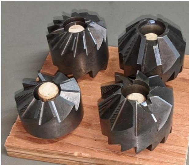
The valve seat cutters were old school tools from the automotive repair industry made by Kwik-Way. Though old school, they are still very effective tools, especially with freshly ground cutting edges. There are a variety of carbide valve seat cutters available these days but they are quite pricey so these were a cost effective option.
