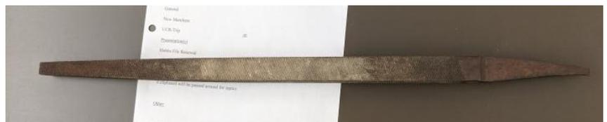
Large files can be sharpened multiple times. Smaller files may only be good for one or two sharpening's, depending on the files style and the degree of wear. Files that are dropped off or sent in can be sharpened and then shipped back.
