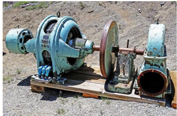
Smaller Pelton Wheel and Generator
