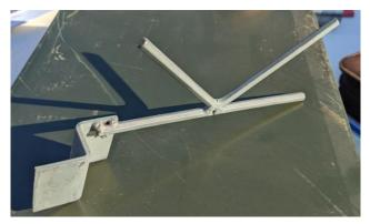
desired weld path. They allowed the user to just lightly slide the rod along while welding. It allowed him to better focus on maintaining the desired weld puddle since he no longer had to focus on the path of the weld. He had some
