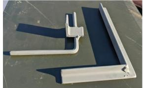
that were optimized for miters and some for straight joints. One was set up for long straight beads. They could be used for stick or MIG and could also be applied to cutting processes.
