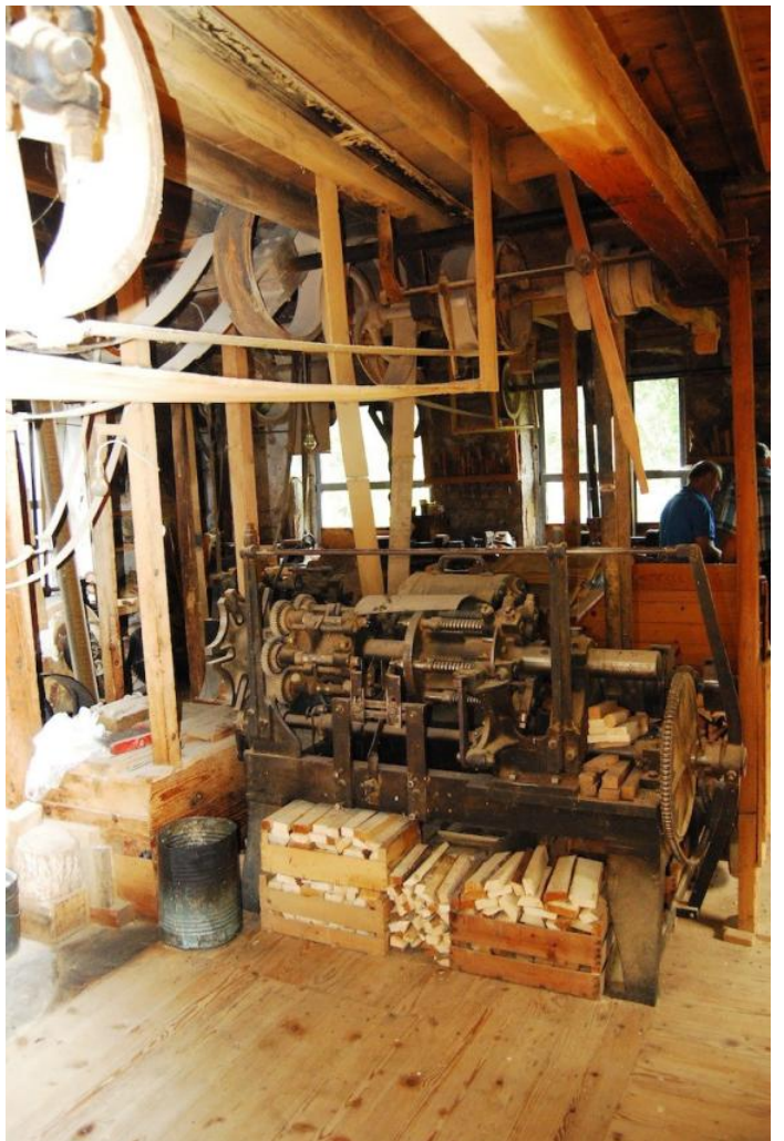
Complex Line Shaft and a Turret Production Machine
