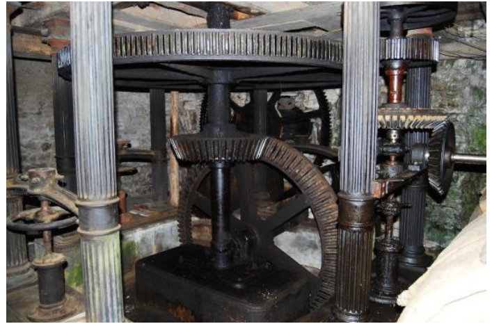
Giant Gear Assembly for Distributing Power
