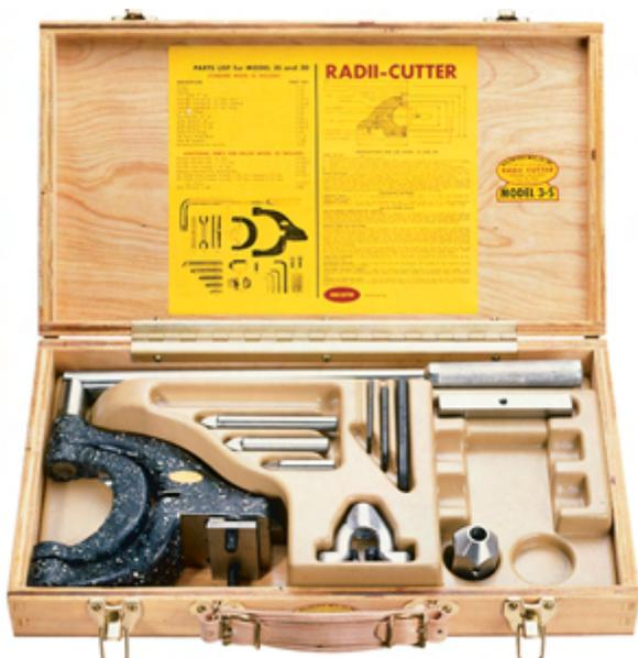
myriad of adjustments and can accurately sharpen twist drills from 1/8th to 5/8 diameter. It demonstrates the offcenter conical rotation necessary to put the proper clearance on the drill point lips.
