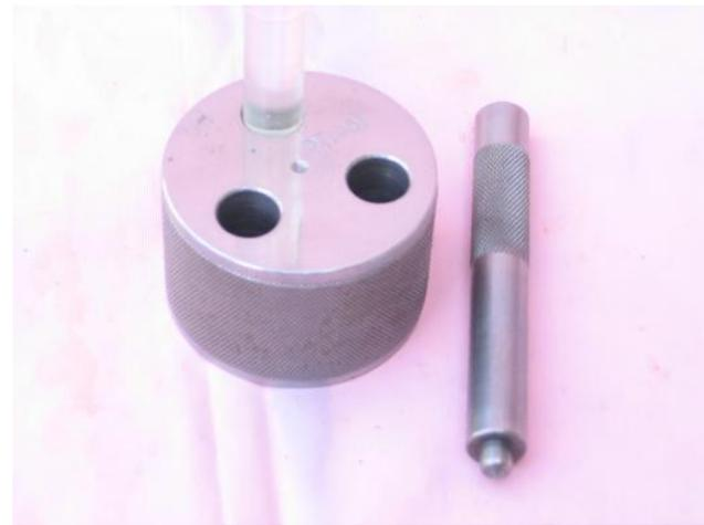
The Lucite rod is placed in a hole and is used to visually locate the center of the hole over the target layout lines. Once located the Lucite rod is removed and replaced with a center punch and a punch mark is made. The accuracy of the device depends on the accurate location of cross-hairs on the Lucite rod as well as an accurate location of the center punching point.
