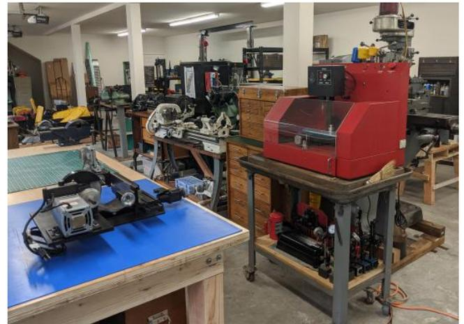
out-of-date motors and electronics. The one setting on the table in the foreground is a CNC cam grinder with a diamond wheel he uses for grinding carbide tooling. It was quite impressive, and I am sure there were more than a few envious viewers during the tour.
