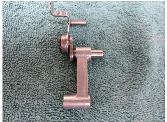
added plenty of lubrication and restored free movement of the part. He then reassembled the mechanism, made a few key adjustments and had a good working machine again.
