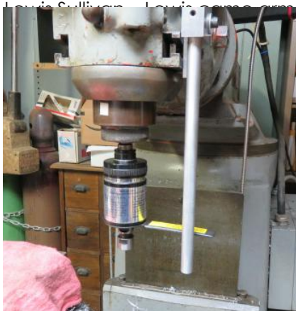
Vertical Bar Mounted on the Mill
