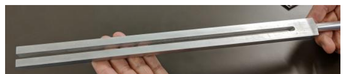
The Finished Large Tuning Fork
