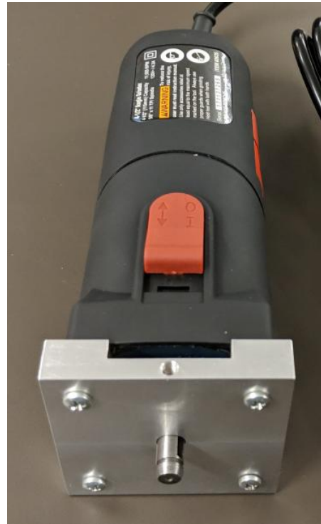
Finished End Plate Mounted to Motor Body
