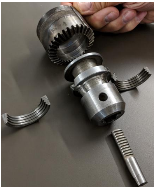
Low Cost Chinese Chuck after Cutting Ring Off
