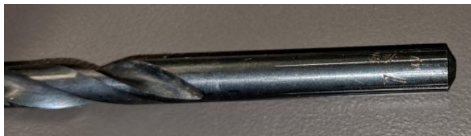
Used Drill Bit Showing the Chuck Jaw Marks from a Keyless Chuck
