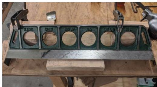
Here is an example of what appears to be a shaper ram. One of Richard's original Kingway alignment tools is shown checking the alignment of the various flat surfaces in an effort to bring them all into parallel planes.
