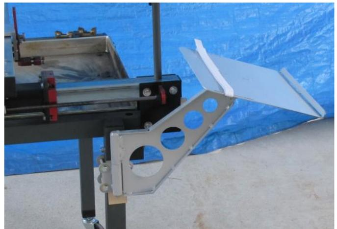
He shared a video of cutting a piece of steel and it was surprising how fast it moved. As can be seen in the photos, the cuts are quite clean. One thing he mentioned was that he adds Borazo to the water under the cutting table. This raises the pH and reduces the tendency to form rust. One last photo shows the table and his laptop during a cutting
