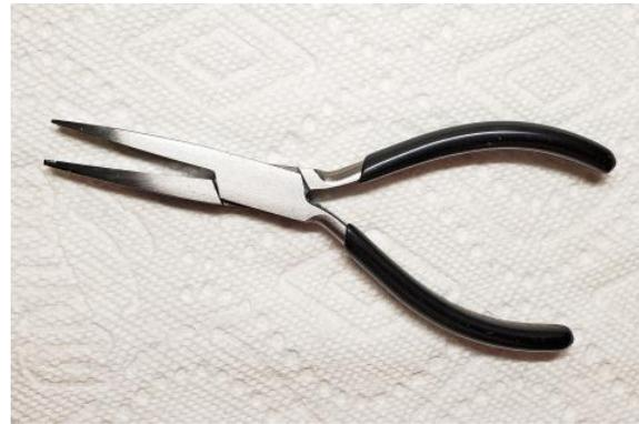
After a few guesses from the group he revealed that they were for removing E-clips. They are specially shaped to grip the back side of the clip so that it remains in one's possession as it is extracted from a shaft. Without these pliers it is not uncommon for the clip to go flying to places
