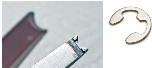
unknown during a typical removal. They are designed for specific ranges of E-Clip sizes.
