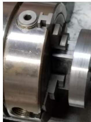
Flywheel Turned In Lathe
