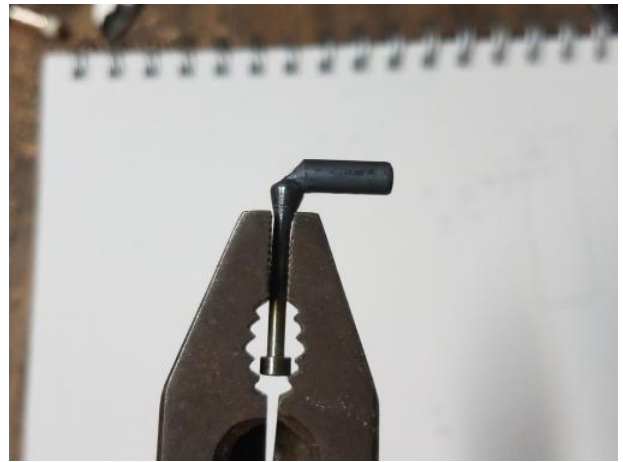
Steel Air Valve After Bending 90 Degrees
