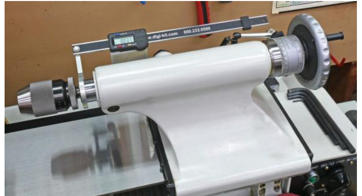
DRO Installed on TS
