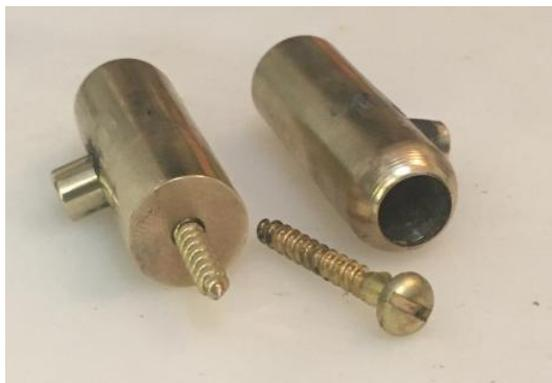
These then were screwed to the underside of some cubbard or cabinet and the two beaters just snapped into place.
