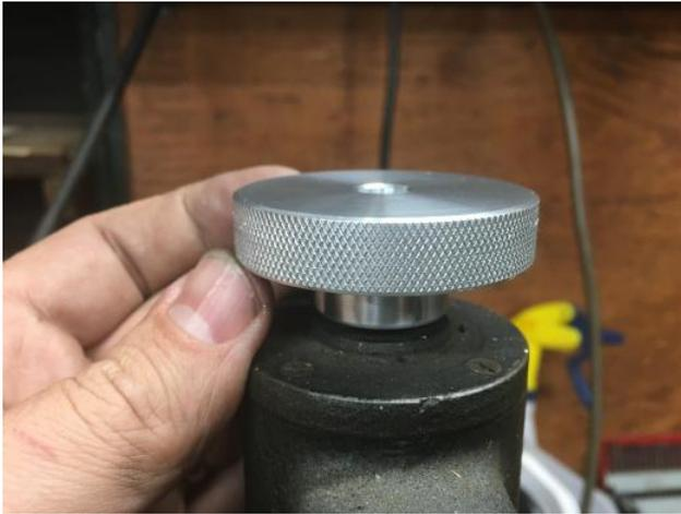
He showed a video of the tool tapping the aluminum knob. It was having a hard time developing much torque, but it did work. The slippage was no doubt due to the condition of the rubber traction cone wheel and the fact that he was not applying much force. This will be a good tool to have.
