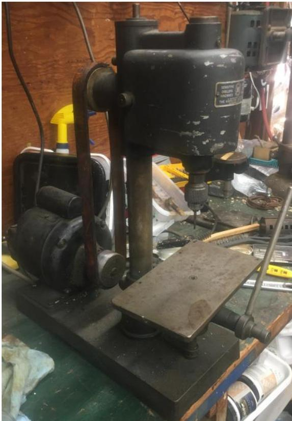
found this tool back East somewhere and had it shipped out here. It was functional with fairly minimal work. Note the rubber drive cone located between two hubs on the vertical shaft. The work is moved up from below with the arm
