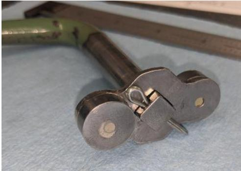
The last image shows the new part mounted in the gear box with one of the round protrusions engaged in the slot of the shifting mechanism.
