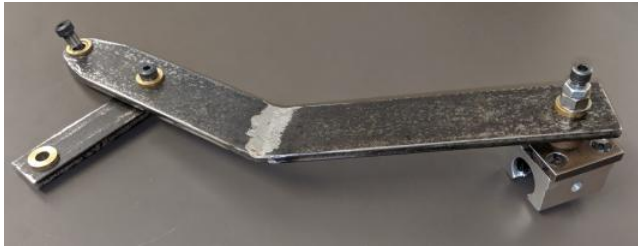
Threading Attachment Sine Bar
